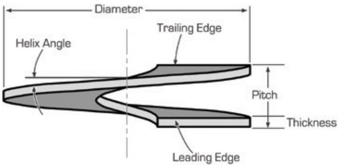
A helix plate is formed by cold pressing the steel plate with matching machined dies. Both the shape of the die press and the amount of applied force during the press operations is important to ensure parallel leading and trailing edges and the required pitch tolerances. The amount of die press force must also be adjusted for changing plate thickness or steel grades.
