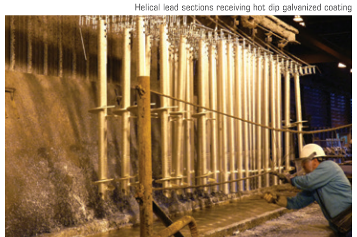
Helical lead sections receiving hot dip galvanized coating
