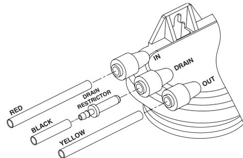
2. Locate the  $\frac{1}{4}$ " Red Feed Water Tubing. Remove the red plug from the fitting labeled "In" on the manifold and insert the tubing. Reference the special supplement sheet in the carton for proper connection of all tubing and removal of plugs. Run the tubing along its course to the Feed Water Saddle Valve, trim to length. (Refer to Fig. 1.)
