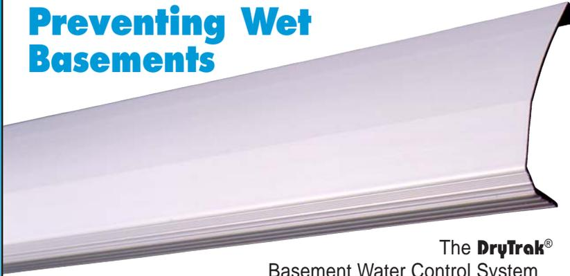
The **DryTrak®** Basement Water Control System combines superior materials and practical design to remove seepage from the troublesome floor-wall joint and direct it to a sump pump or drain. The removal of this water lowers the water table around your foundation, thus relieving hydrostatic pressure. The **DryTrak®** system is very effective on all types of foundations including poured concrete, brick, block, stone, etc.
